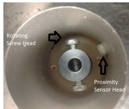
Figure 24 – Proximity Sensor installation [1]
