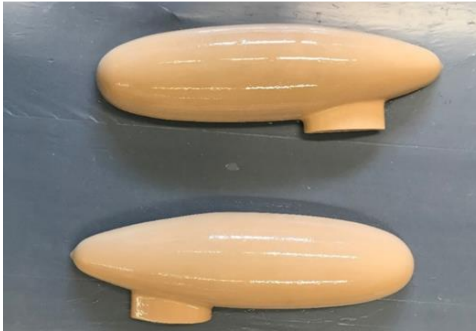
Figure 13 – Machined plug used for vacuum bagging of the nacelle
